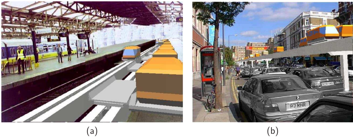
Figure 6: (a) Some of the platforms at Victoria Station have been transformed into carrier exchangers. Here, cabins are automatically unmounted from a road carrier (see Section 1.3.3) and mounted onto a guideway carrier (see Section 1.3.2). (b) The faster high-capacity guideway carriers take cabins to more remote, predominantly suburban destinations. After the introduction of MAIT traffic congestion (in grey) below the guideway may be a thing of the past .
