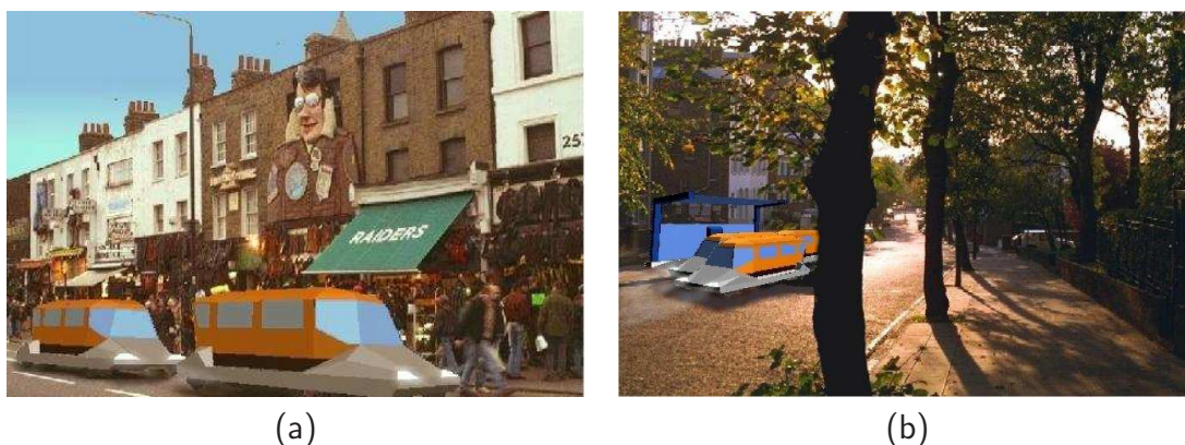
Figure 5: (a) Road-carrier with wheels and tires in Camden, UK. Here, people share the road with MAIT vehicles. Even though it only travels at walking speed the road-carrier must be equipped with infra-red and ultra-sonic sensors to detect obstacles. Slow speeds are not a drawback since the trips with this carrier type are usually short. (b) Road-carrier vehicle is passing by an off-line stop with shelter on a low traffic density street in London.
